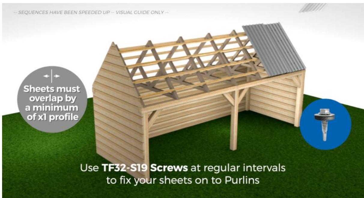
It's important to allow the sheets to extend beyond the bottom purlin to enable rainwater to effectively drain into the gutters below or fall beyond the below wall.
